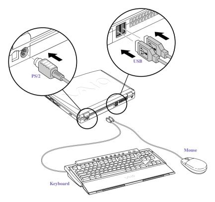
To connect both a PS/2 mouse and keyboard at the same time, use an optional PS/2 division connector.
